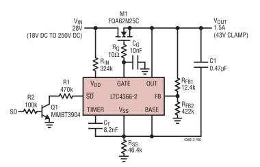
Figure 6. Overvoltage Protected 28V, 1.5A Supply
