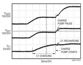
Figure 2. Turn-On Waveforms
