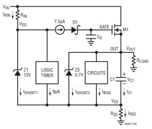
Figure 5. Simplified Block Diagram
